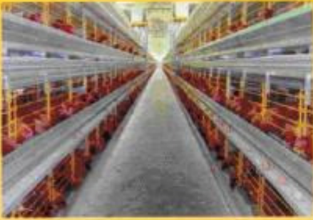
Battery type poultry cages with automatic feeding trolley & automatic egg collection
